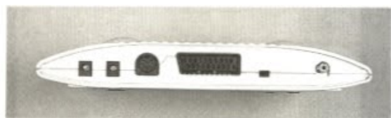
From left to right: 5 Volt power connector (dangles from appropriate Amstrad monitor), 9 Volt power connector (for use with supplied power pack), A/V monitor connector (the one that won't work with old-style CPC monitors), SCART socket, sound on/off switch, TV connector.
