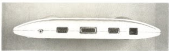
From left to right: stereo phono socket, player 1 joypad/joystick connector, analogue joystick port (accepts two sticks with suitable adaptor), player 2 joypad/joystick connector, auxiliary port for light gun.
