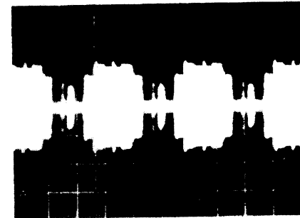
⑧ 20uS/div 10mV/div Mode : REC Test Tape : Blank Tape HIC101 Pin 18
