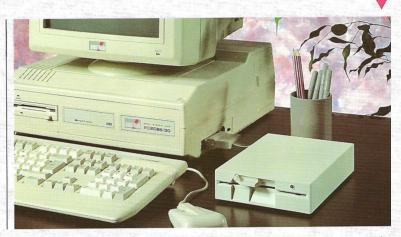
he resolution of a display screen is an important element in the overall quality of a system, particularly when the user may be working at the screen for several hours at a time. The key indicator of this is the dot pitch, which in a quality, high resolution monitor will be a low figure, increasing as the resolution decreases. Within the Amstrad monitor range a dot pitch figure as impressive as 0.28 may be attained.
