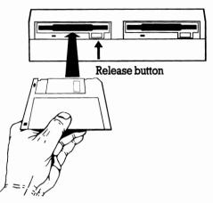
Note: If the instructions tell you to put a disk in Drive A, this means your floppy disk drive -or the drive nearest the keyboard if you have two floppy disk drives. The floppy disk drive furthest from the keyboard on a two-drive PPC is referred to as Drive B.
