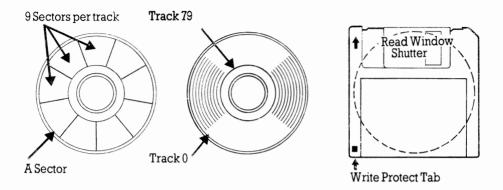
The first thing to notice about a  $3^{1/2}$  inch floppy disk is that it has an upper and a lower side. The upper side has the manufacturer's label on it and a small arrow imprinted in the plastic casing. On the lower side can be seen the metal driving hub, in the centre, and a plastic 'write protect' shutter in one corner. Disks are always put into the AMSTRAD PPC's drives with the arrow uppermost and pointing away from you.
