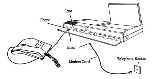
The AMSTRAD PPC modem is designed as an integral part of the PPC. There is nothing for the user to connect up, except for thephone line which is unplugged from its socket and plugged into the socket labelled "PHONE" at the rear of the PPC. Using the telephone extension cord provided, complete the telephone connection by plugging one jack into the socket labelled "LINE" at the rear of the PPC and the other into the telephone wall socket (this prevents loss of normal phone use).
