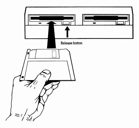
If the drive appears to be resisting the disk, stop. Check that there is no obstruction in the drive. Make sure that you have the disk the right way up, and try again. If you still have problems inserting the disk, consult your dealer. Whatever you do, don't force the disk into the drive.
