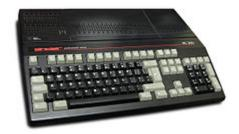
In late 1988 Amstrad created a desktop computer based on the PPC design, intended for the home market. The LCD was replaced by an <a href="RF">RF modulator</a> to display CGA video on a domestic television, and the keyboard and system unit were combined in an integrated case
