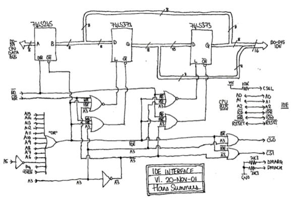
The IDE registers are mapped to eZ80 I/O addresses in the range &0020 to &002F. The high byte is written or read on port &0028. When writing a byte, the high byte register must be written prior to writing the low byte (&0020) so that it is available for sending to the disk drive, which occurs on writing to &0020. Similarly, reading from port &0020 reads the low byte and latches the high byte from the disk drive, which can then be read from port &0028.
