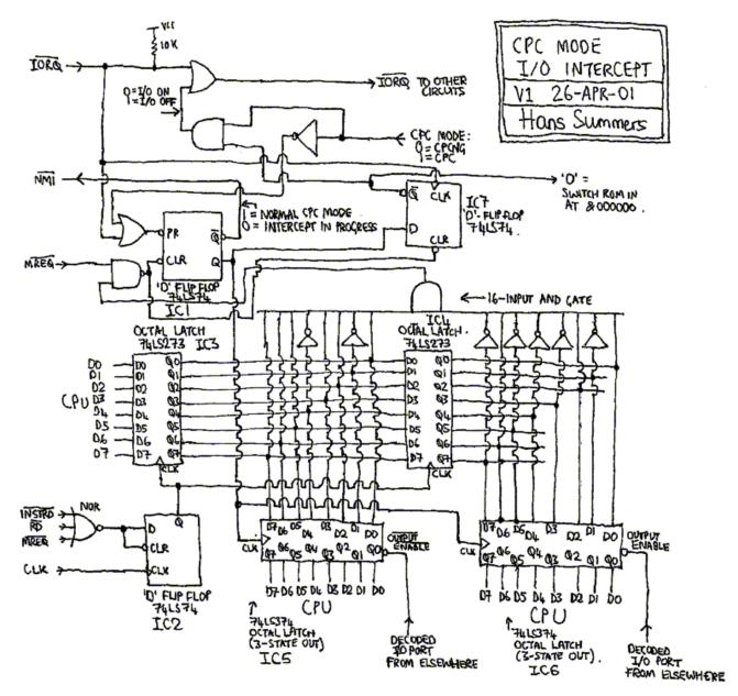
The signals at the left of the diagram connect directly to the eZ80 CPU. At the top, the /IORQ signal from the CPU goes only to this circuit, not to any I/O devices in the rest of the CPCNG.
