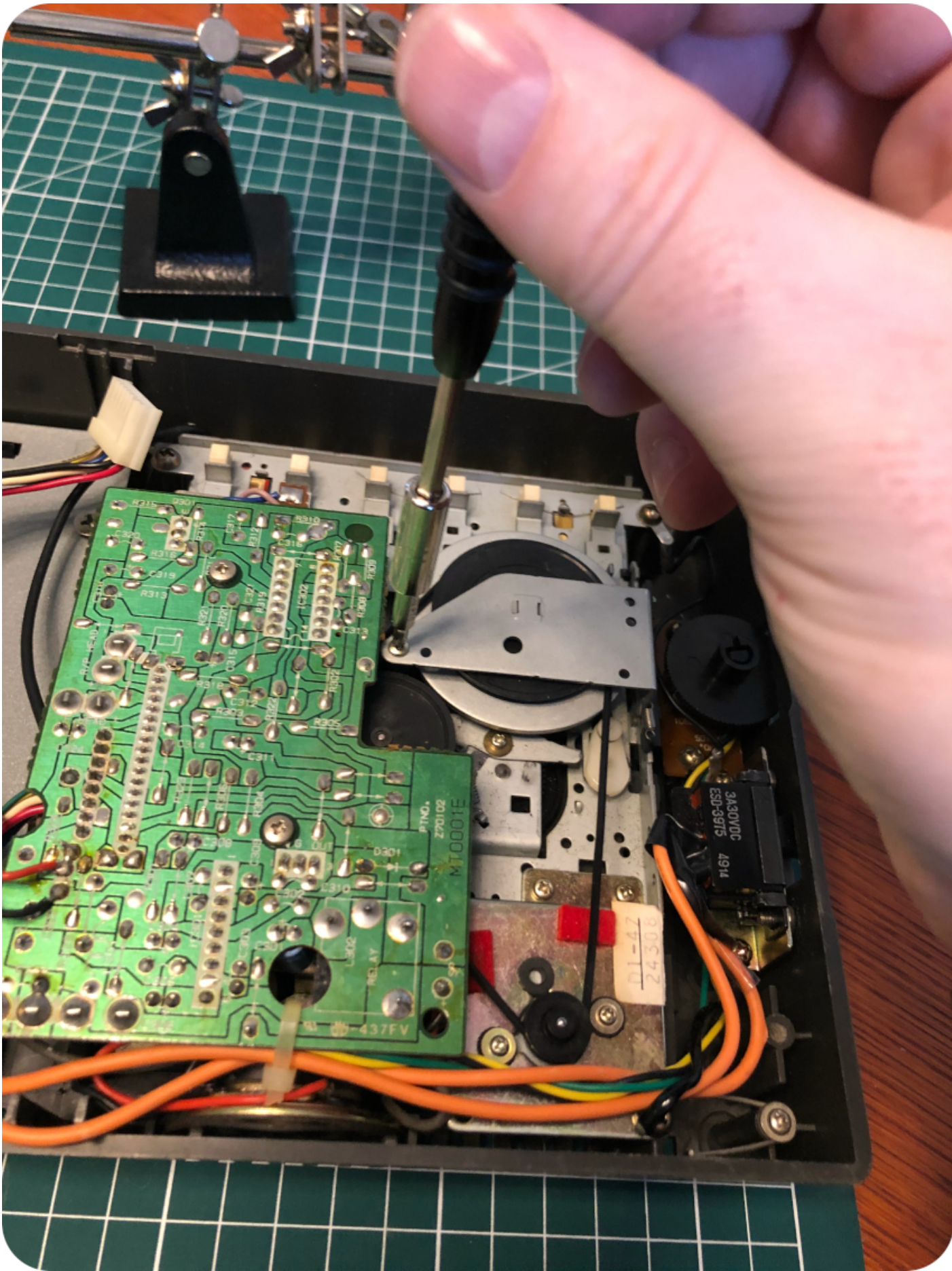
Then pull off the belt from the cog and slide it underneath the metal plate :
