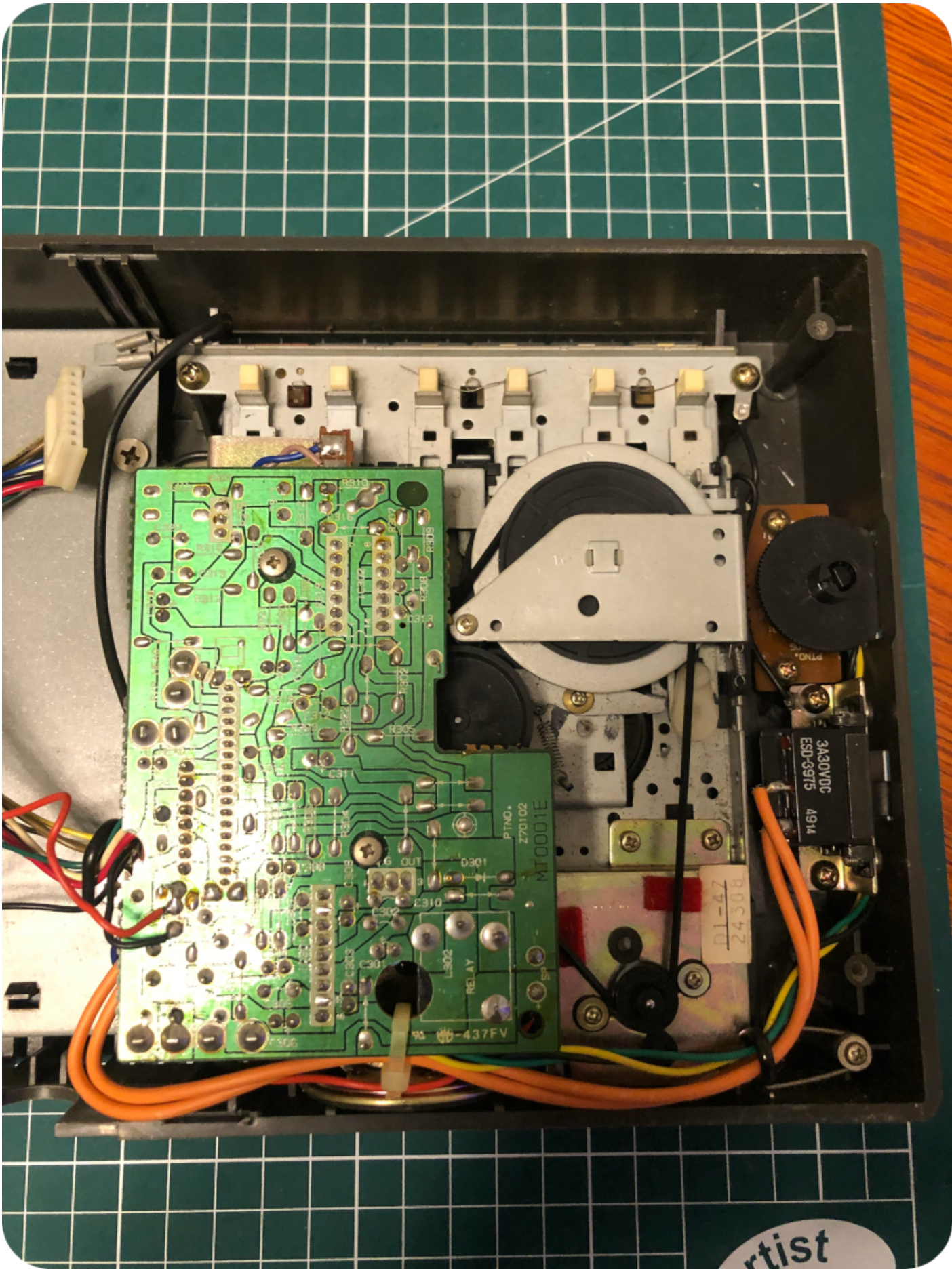
Inspecting and cleaning the PCB
