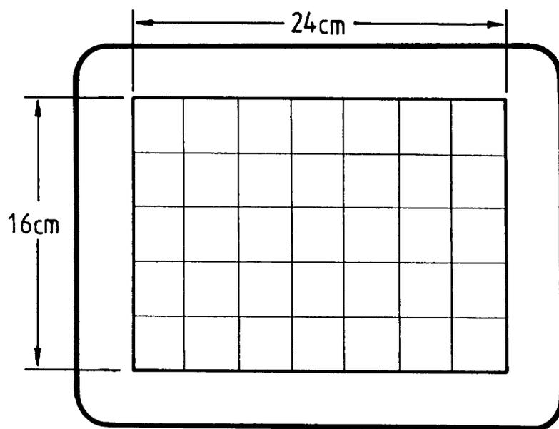
Display Measurements Using the Crosshatch Pattern on the Colour or Monochrome Monitors.
