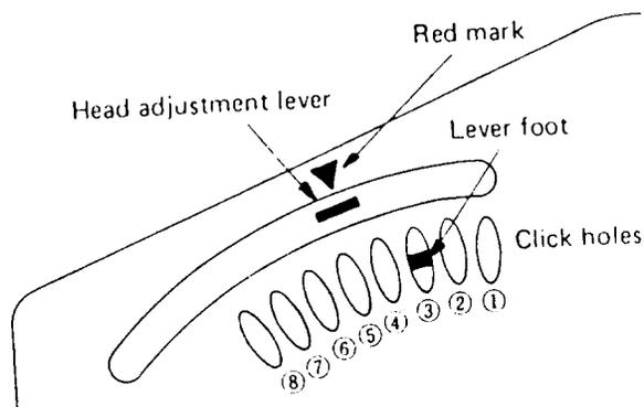
The settings graduate from position 1 for very thin paper, to position 8 for thicker paper. Position 3, indicated by a red arrow above the Head Adjustment slot, is suitable for general purpose computer paper, including Amsoft Printer Paper.
