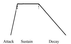
The Sound Manager allows two types of envelopes; amplitude envelopes to control a sound's volume and tone envelopes to control its pitch (the pitch is varied in much the same way as the volume). The user can set up to 15 different envelopes of each type. The exact formats of the data blocks specifying envelopes are given in SOUND AMPL ENVELOPE and SOUND TONE ENVELOPE.
