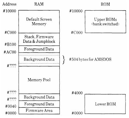
The sizes of the two background areas depend on the background ROMs fitted to the machine (see section 10).
