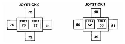
Note that joystick 1 overlays keys 48..53 on the main keyboard and is indistinguishable from them.
