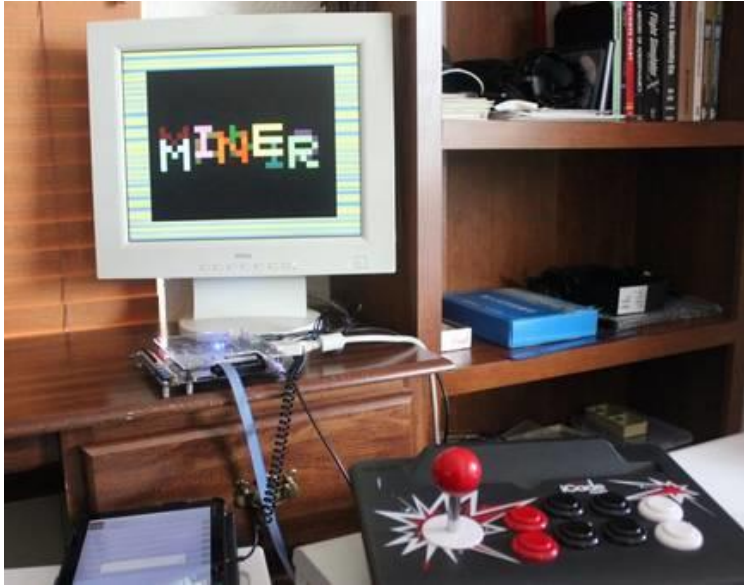
Image 3 : Sinclair ZX Spectrum on Altera DE1
