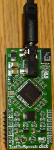
EPSON S1V30120 "TEXT TO SPEECH" CLICK DAUGHTER BOARD FROM MIKROELEKTRONIKA
