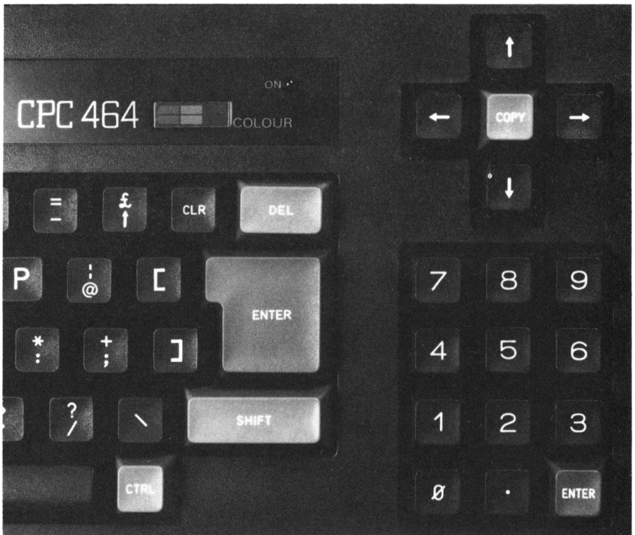
Fig. 2.3 Keys involved in EDITing programs: cursor position, COPY, CLEAR and DElete keys.
