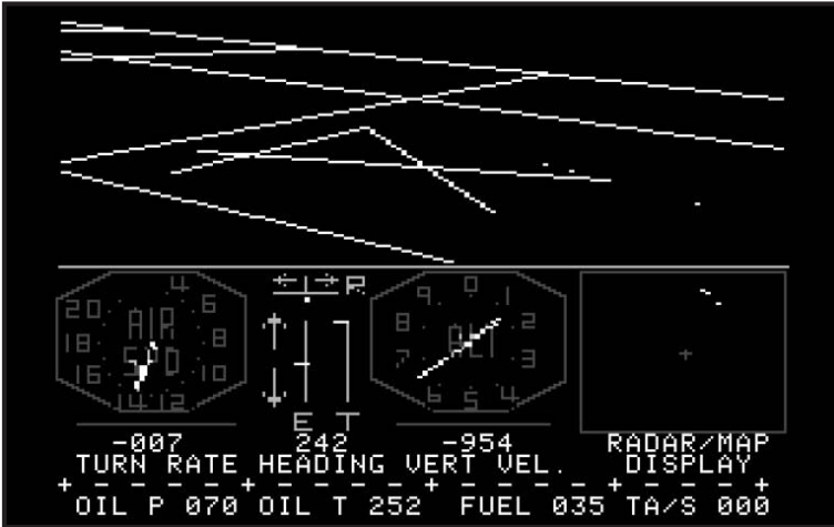
The original Flight Simulator . The cockpit view was updated only about 3 to 5 times per second.
