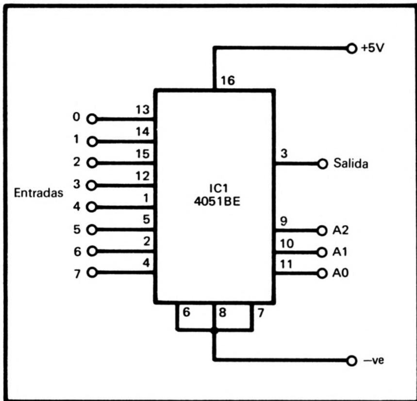
Figura 38.—Multiplexor/demultiplexor analógico CMOS
