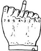
$$\begin{aligned} &= 16 \text{ decimal} \\ &= 10 \text{ H hexadecimal} \end{aligned}$$
