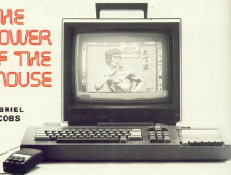
If you still think a mouse is just a furry mammal you haven't been keeping up with hardware developments over the last few years. A mouse is also a small plastic box with one or more buttons on top, and a tracker-ball mechanism underneath.
