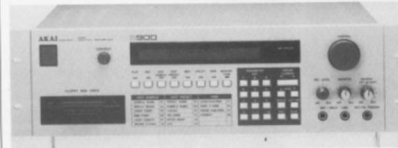
Akai's S900 - 12-bit sampling from 7.5kHz to 40kHz. Maximum sampling time is just over a minute.
