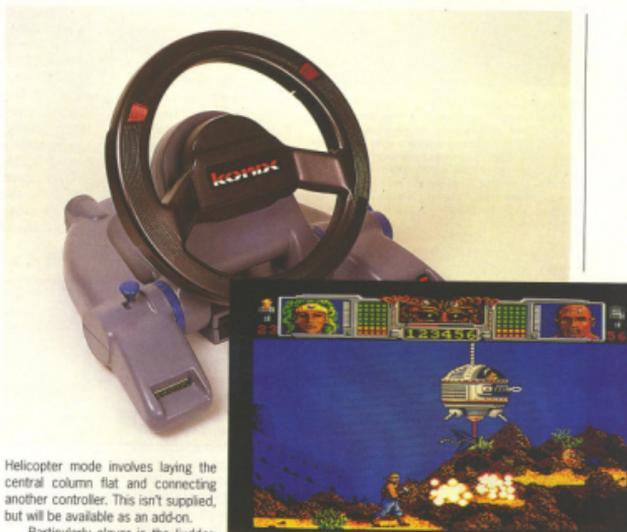
Helicopter mode involves laying the central column flat and connecting another controller. This isn't supplied, but will be available as an add-on.
