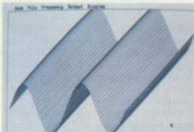
**Replay Professional** - no, it's not Origami with graph paper but a three dimensional display (fast Fourier transform) of a sine wave sample.
