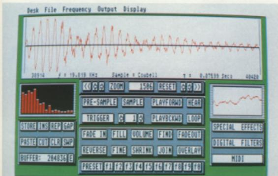
The main control screen of **Replay Professional**. The main sample covers the upper half of the screen whilst a harmonic analysis is displayed on the lower left and filtering characteristics on the right.
