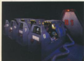
Each cockpit is equipped with a 23" colour monitor, which serves as a front window to the vehicle and displays graphics of the surrounding environment and the ensuing battle. The secondary screen is used for radar and vehicle status. Dual joysticks with trigger buttons, weapon selection displays, throttle control, directional pedals, ceiling message centre, radio communication with team-mates and attendant and other interior battle functions all add to the realism of the battle
