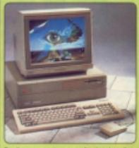
For the more serious or professional applications user, Commodore have a selection of systems based around the expandable Amiga 2000, at prices from £1295-VAT. The A2000 features a full 1MB RAM (expandable to 8MB), 19 system expansion slots, plus IBM compatibility with the use of PC-XT or PC-AT intelligencers. Complete and return the coupon, putting a tick in the A2000 box, for details of A2000 computer systems.
