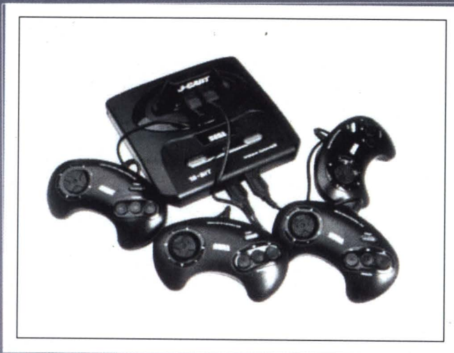
The J-Cart, Codemasters' ingenious sidestepping of the limitations of two joypad ports. By plugging extra pads into the cartridge, the player count could effectively be doubled
