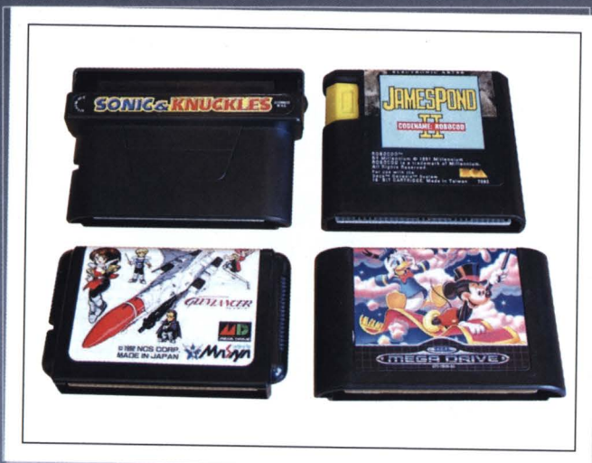
From top-right, clockwise: EA's standard oversized cartridge, with useless yellow tab; a UK example, the standard 'mushroom' shape; a Japanese cart, with rounded edges and cutaway; and Sega's Sonic & Knuckles , with its connector for mounting any other Sonic title
