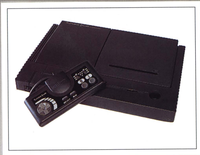
As the first of the PC Engine superconsoles containing all the hardware of the HuCard and CD-ROM units in one machine, there is no need for system cards with the Duo
