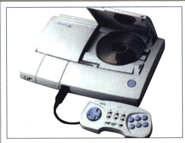
The final PC Engine Duo, the Duo-RX, comes complete with a six-button pad almost identical to that seen in NEC's Japan-only PC-FX console
