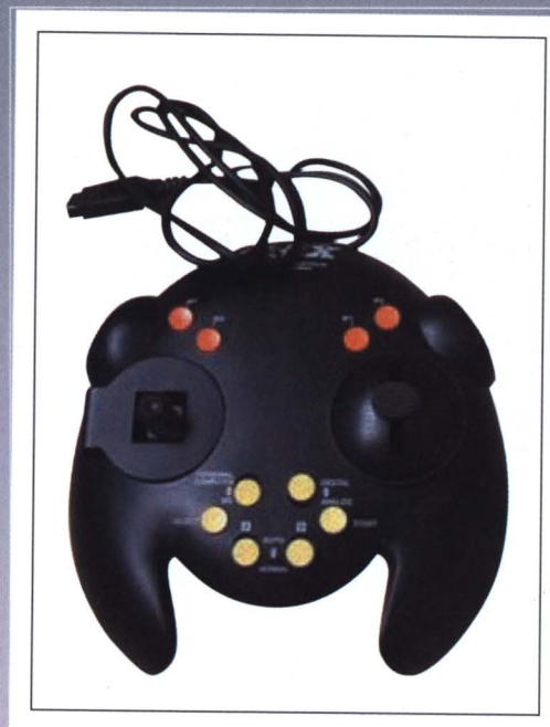
Long before Nintendo's N64 effort came the AX-1E Analogue Pad, complete with variable-rate triggers and thumbsticks. A very similar looking pad was later released for Sega's Saturn console
