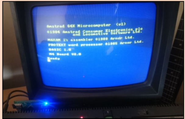
THE START UP SCREEN WITH THE M4 BOARD INSTALLED AS WELL AS VIRTUAL MAXAM AND PROTEXT ROMS
