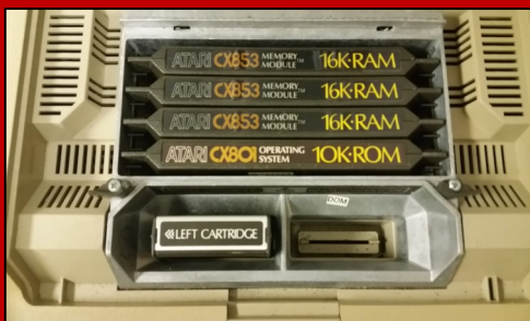
THE ORIGINAL ATARI 800 HAD USER-ACCESSIBLE EXPANSION SLOTS FOR RAM AND ROM CARDS AS WELL AS LEFT AND RIGHT CARTRIDGE PORTS.
