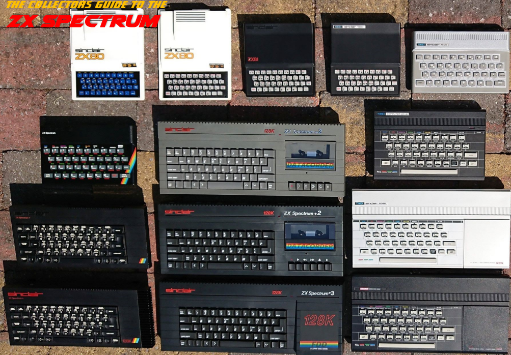
SINCLAIR AND IT'S TIMEX COUSINS. THE BOTTOM RIGHT MICRO IS A POLISH UNIPOLBRIT KOMPUTER 2086 WHICH IS BASICALLY A CLONE OF THE TIMEX SINCLAIR 2068.
