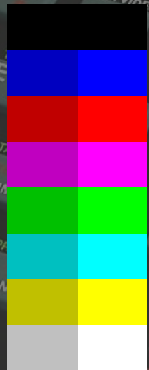
THE ZX SPECTRUM CAN DISPLAY 8 COLOURS AND 15 USING THE 'BRIGHT' ATTRIBUTE. THE 'BRIGHT ATTRIBUTE' COLOURS ARE THE ONES ON THE RIGHT IN THE GRID ABOVE. 'BRIGHT BLACK' IS STILL BLACK SO THAT'S WHY THERE'S 15 COLOURS INSTEAD OF 16.
