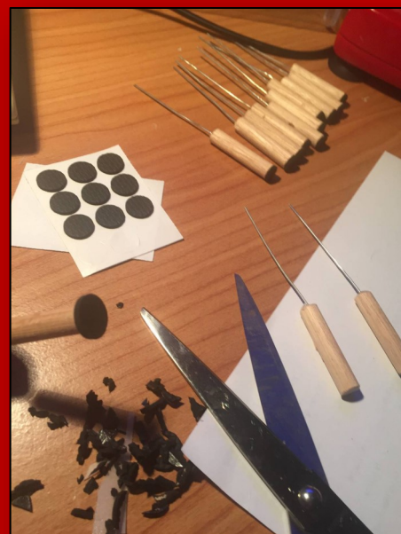
For the 'fret fingers' I cut wooden dowel, drilled a small hole in one end of each and glued a straightened out paper clip into the hole. At the other end I glued rubber feet (that had to be trimmed down a bit with scissors).
