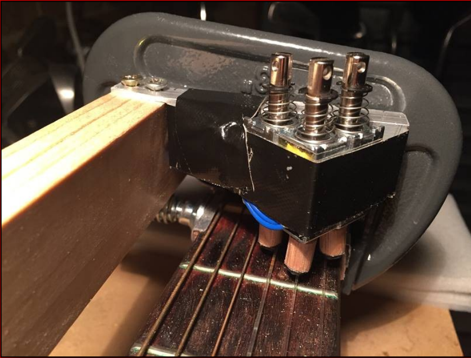
Here is a test I did with 3 solenoids that proved to be unsuccessful. While they moved quickly down to the strings when powered on, the pressure was simply too light and the note when played sounded very muffled. I abandoned this idea and switched to using servo motors instead.
