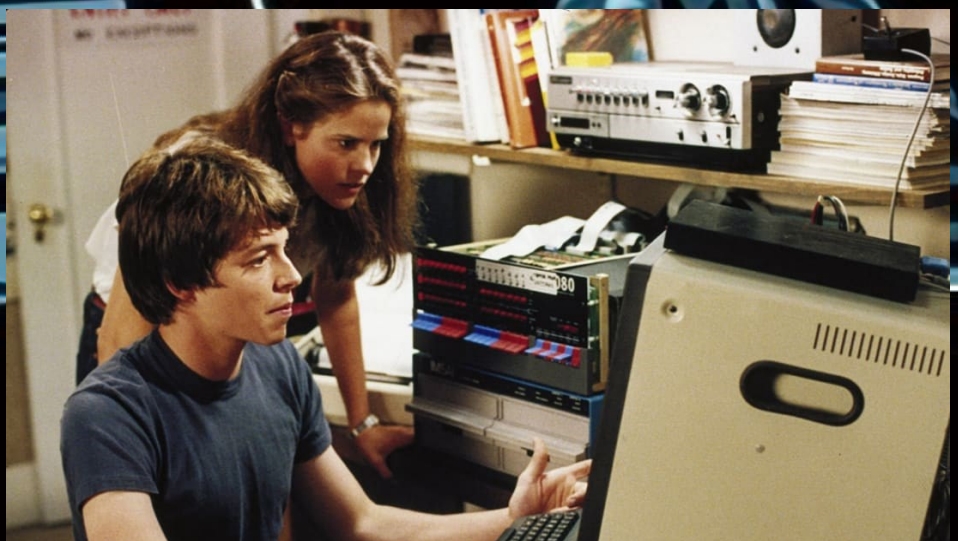
Here you can see the ISMAI 8080, along with it's dual disc drives and 17 inch Electrohome screen
