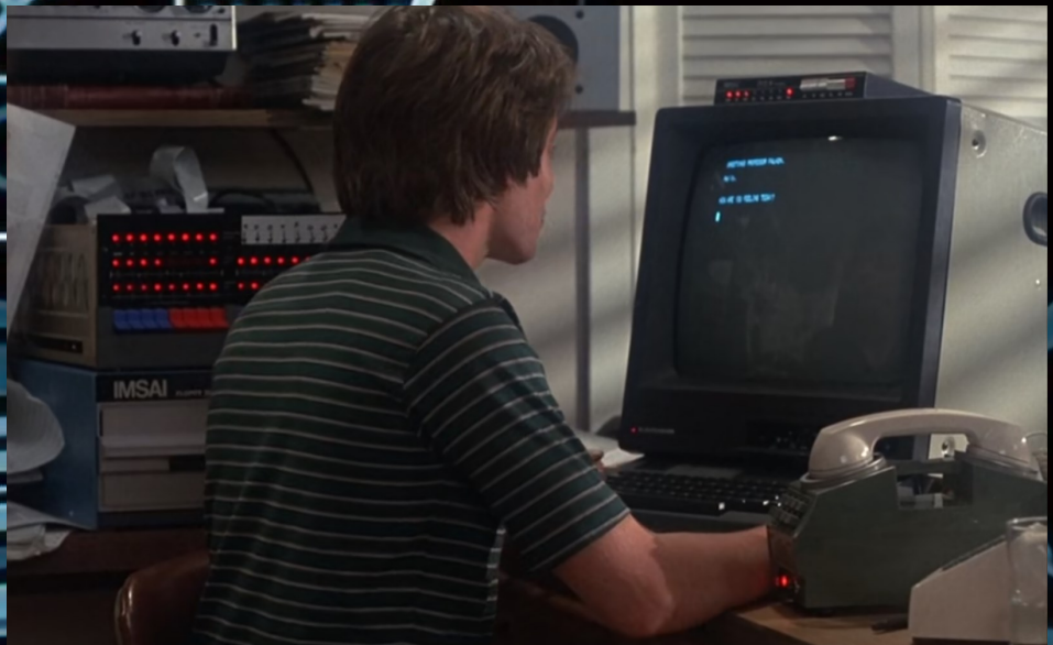
The IMSAI 212 A modem on top of the monitor and the acoustic coupler at the bottom right
