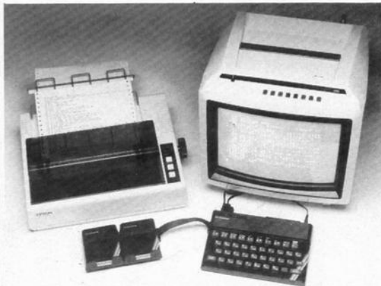
Here the ZX Interface 1 links the Spectrum to two Microdrives and an Epson printer
