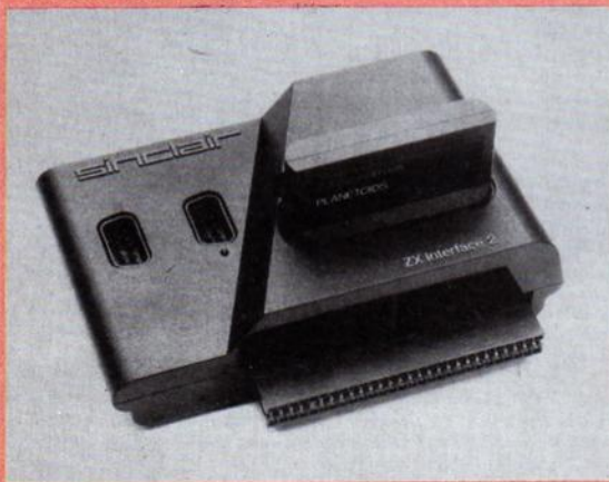
Close up of the Interface 2 — that edge connector might cause trouble in the long run
