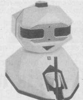
FRED — 12in high and moves at 5in per second
