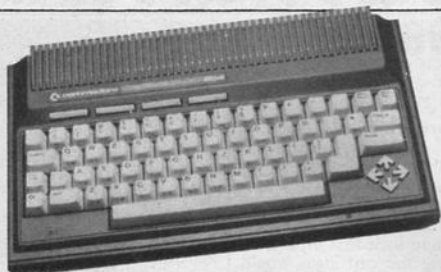
Commodore's C264 — with four wide function keys above the keyboard and arrow-shaped cursor keys set in a diamond shape
