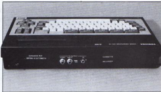
● Rear view showing expansion bus, video, audio and RF output and cassette port. Joystick sockets are on the side and cartridge slot is on the top.
