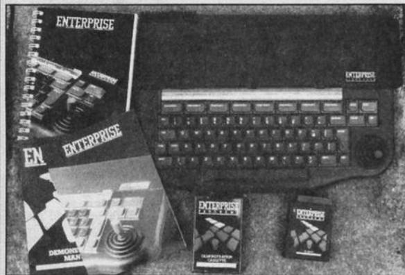
The **Enterprise 64** is one of the very latest micros to appear on the home market. It combines many features not found together in one small package. For example; stereo sound, 256 colours, built in joystick, wordprocessor, 64k memory — expandable to 4000k!
