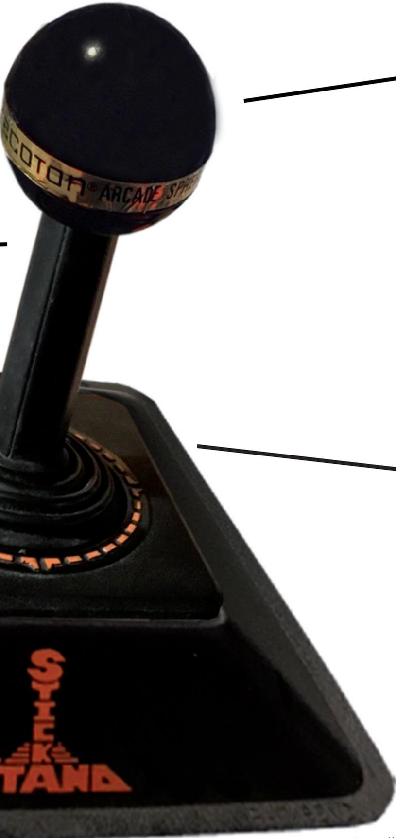
*Get a grip: This Arcade Sphere Ball would go on top of your joystick, allowing for a firm grip like in the arcade. It was just a piece of plastic, though. If anything, it made it much more likely to break your joystick by pushing to hard in one direction.*
