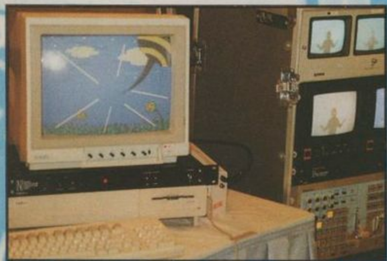
■ The main Eat A Bug control unit where animated Amiga graphics, running on an Amiga 1000, combine with video images of the player to produce a truly interactive game. Let's get swatting!!
