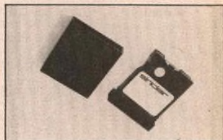
Each Microdrive cartridge (shown here with case) can store up to 50 files — with an access time of 3.5 seconds.
