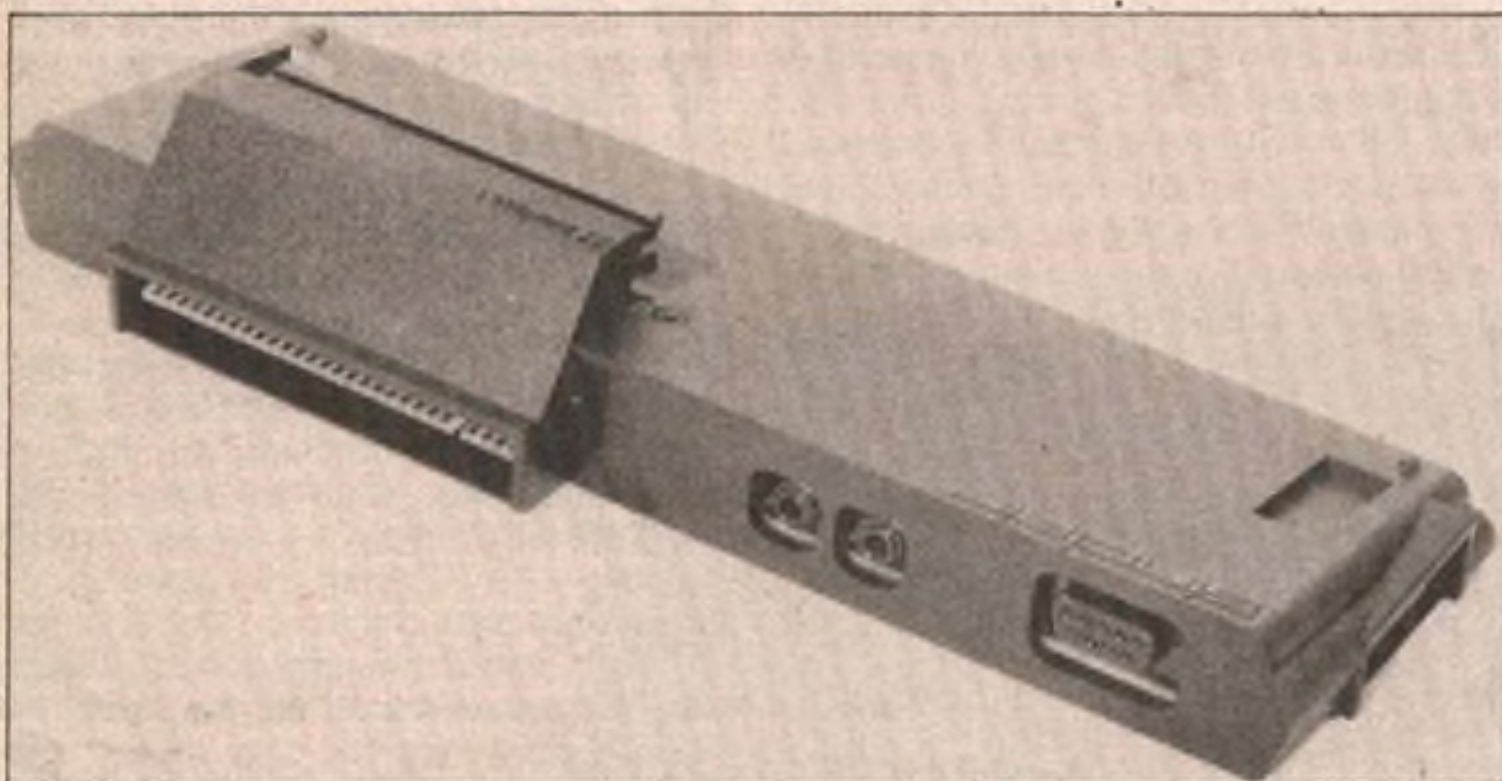
The ZX Interface 1, which fits underneath the Spectrum, operates at all standard baud rates up to 19,200 with speed software selectable.
