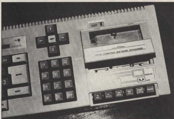
Detail of numeric keypad, cursor controls and built-in cassette unit
