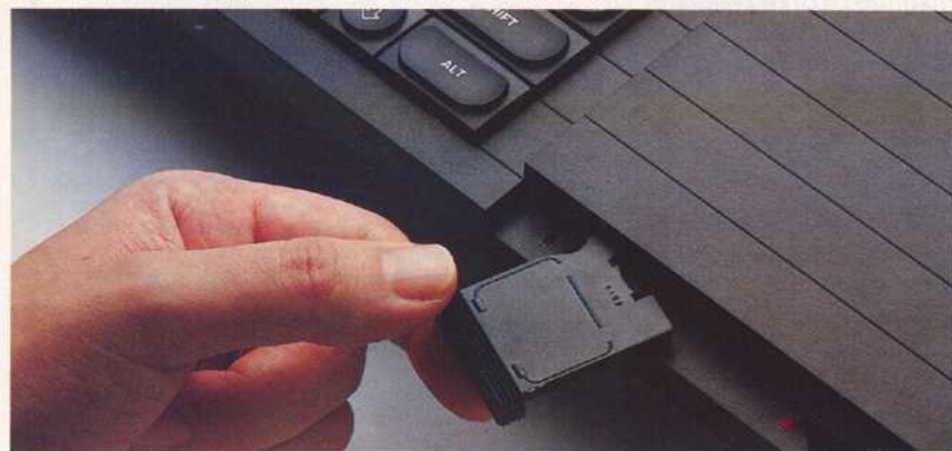
Sinclair Microdrive cartridges - up to 100K of programs and data on a medium so compact you can pop it into your pocket.
