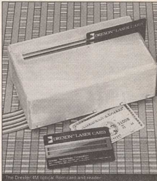
The Drexler 4M optical Rom card and reader
