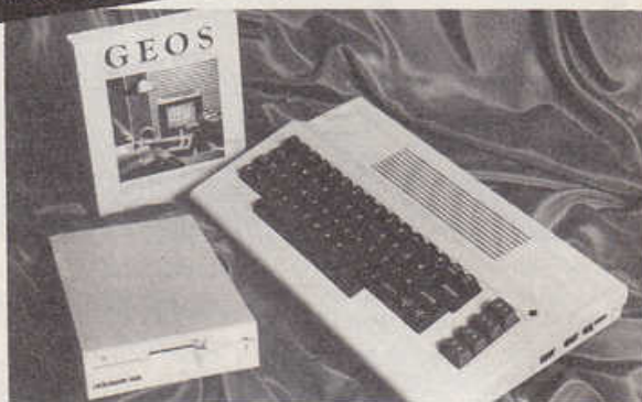
The Excelerator+ & GEOS pictured with a '64 installed in a Slimline case
