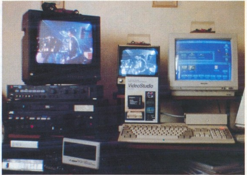
Our reviewer's complete titling set-up with two video recorders and TV/monitors, video camera, Genlock and Amiga with monitor.
