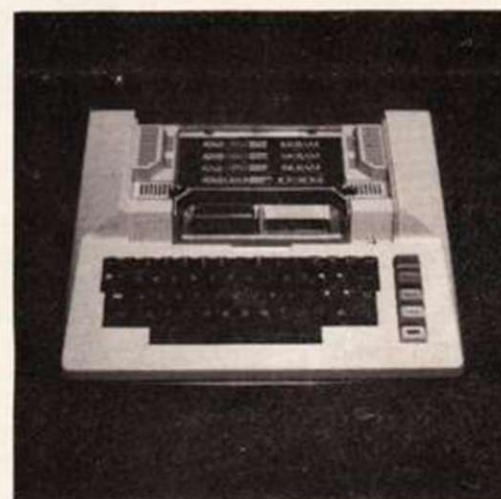
Atari 800 Console (with cover removed)
