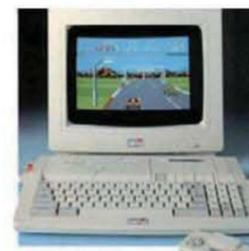
» A new case and the addition of a cartridge slot – for expensive £30 games – transformed the 464 into the 464 Plus
