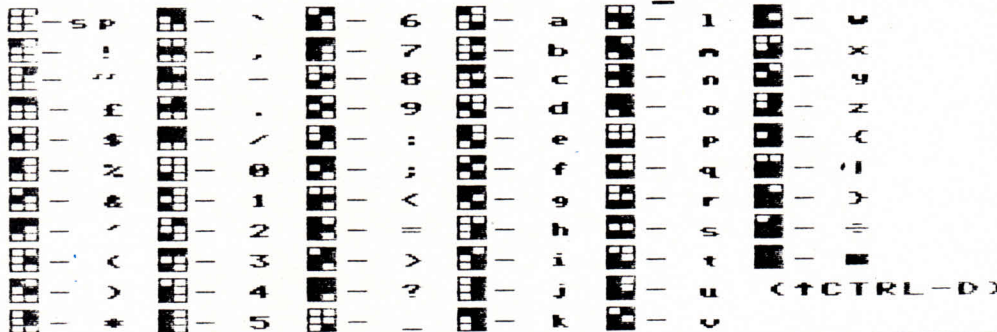
FIG 1- THE VIDEOTEX GRAPHICS MOSAICS. THESE SIMPLE BLOCKS CAN BE USED TO FORM QUITE COMPOSITE PATTERNS ON A VIDEOTEX SCREEN IN UP TO SEVEN COLORS.
