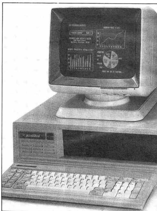
Most of the features of President Computer's new IBM PC workalike are not shown in this photograph. It comes with 512k of RAM (which is expandable to 1024k), an 'intelligent' video display card (combining colour and mono modes under software control) and up to two 320k floppy and two 10Mb hard disk drives all inbuilt into the main cabinet. A portable version of the above with the exception of a limit of one hard disk is also available.
