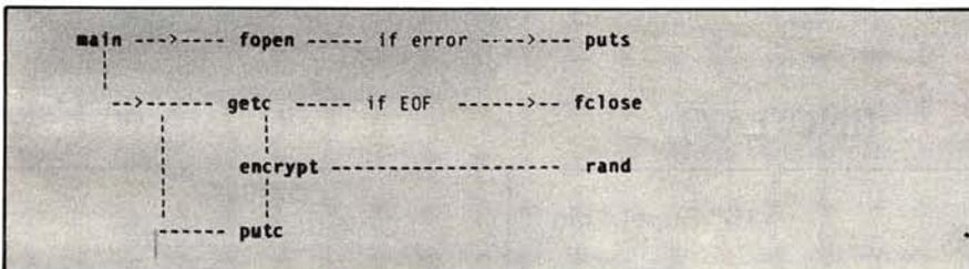
Fig 3 Structure for file encryption program
