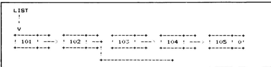
Fig 5 Insertion and deletion by manipulating pointers
