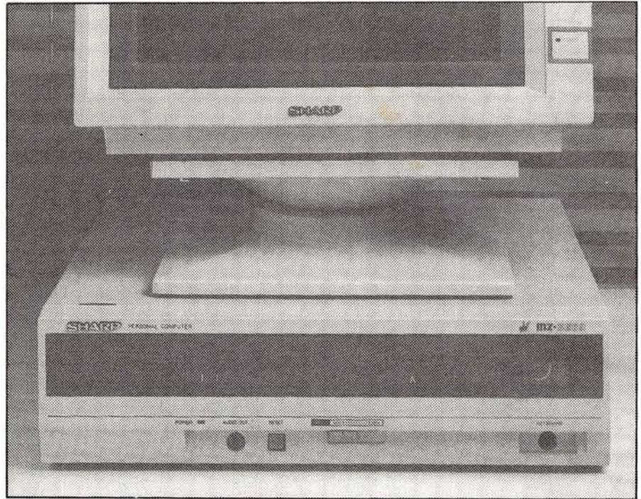
*The front of the processor houses audio output, hard and floppy disks*
