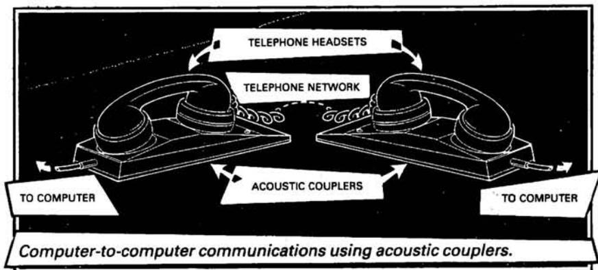
Computer-to-computer communications using acoustic couplers.
