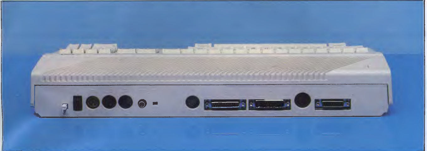
The 520ST is well-endowed with I/O facilities — including a MIDI synthesiser port
