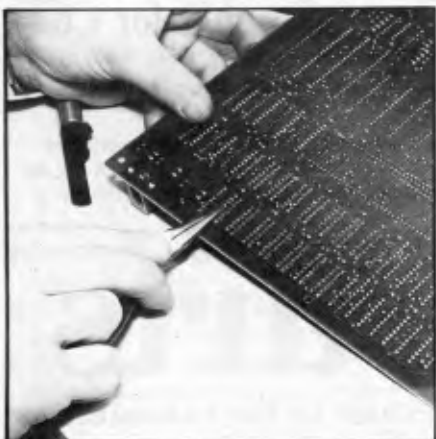
Fig 9 Straightening the IC pins
