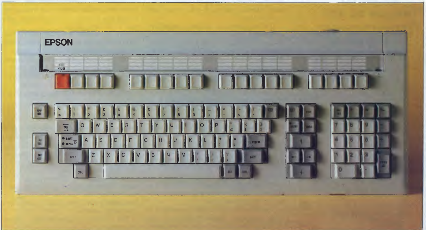
The keyboard sports an impressive 105 keys grouped in a fairly standard manner
