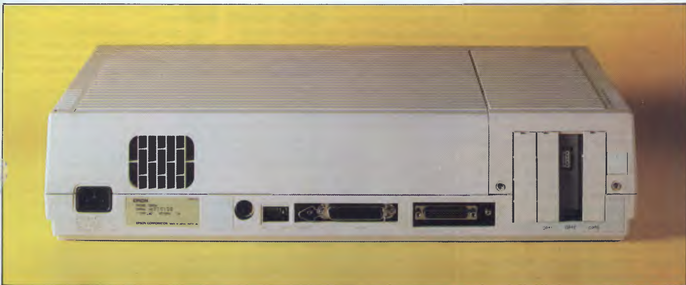
The rear panel has space for four expansion cards but the PCB will only support three
