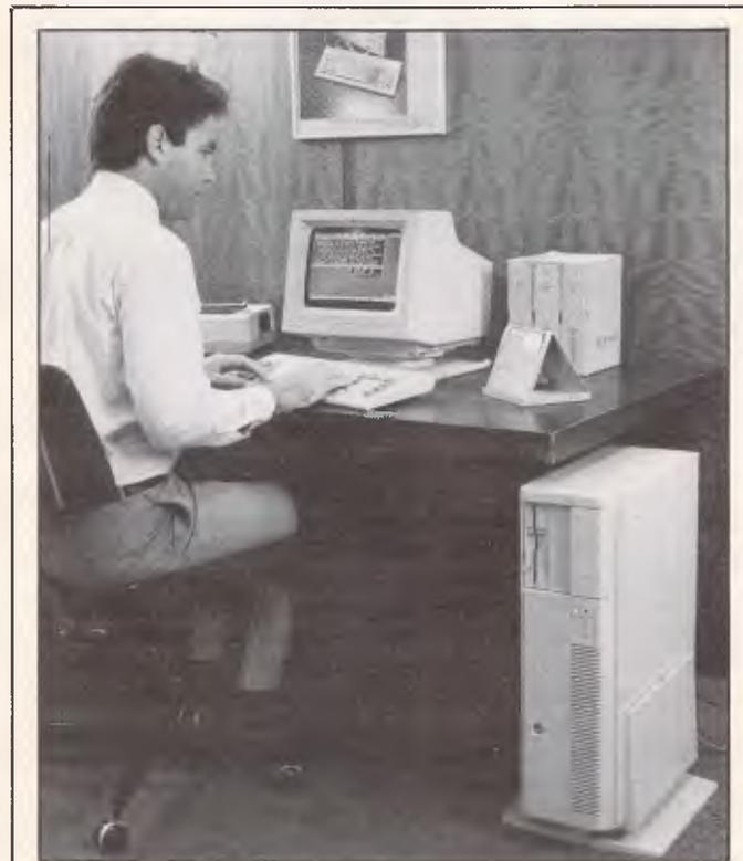
*Sperry is yet another contender in the PC/AT compatible stakes. Its recently announced PC/IT is based on the 80286 processor (the same used on IBM's PC/AT) and comes with half a megabyte of RAM, eight expansion slots and two serial and one parallel port. Up to eight terminals can be attached to the IT.*
