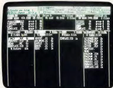
The built-in LocoScript word processing software is amongst the most powerful available and includes such features as pagination, simultaneous editing and printing, automatic paragraph realignment, automatic document editing and reformatting and simple cut & paste editing.
