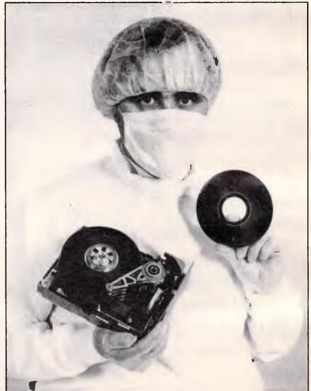
*The IBM PC/AT has a hard disk, which you can't see inside. This picture shows the inside, which can only be opened up in a room with air so clean that even a smoke particle would feel conspicuous.*
