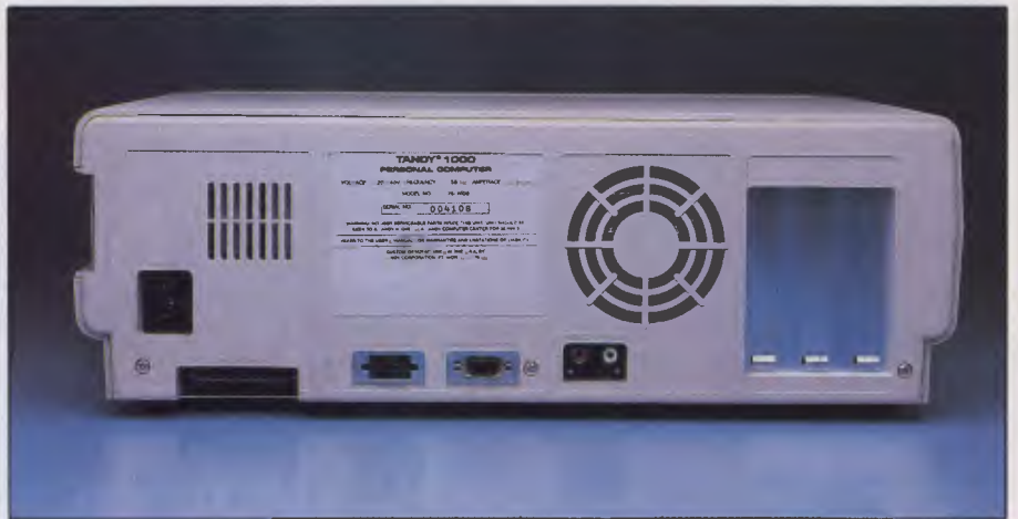
Three expansion slots are on the back of the Tandy
