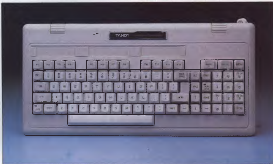
Tandy's keyboard has 90 keys, and is laid out in a non-standard fashion.
