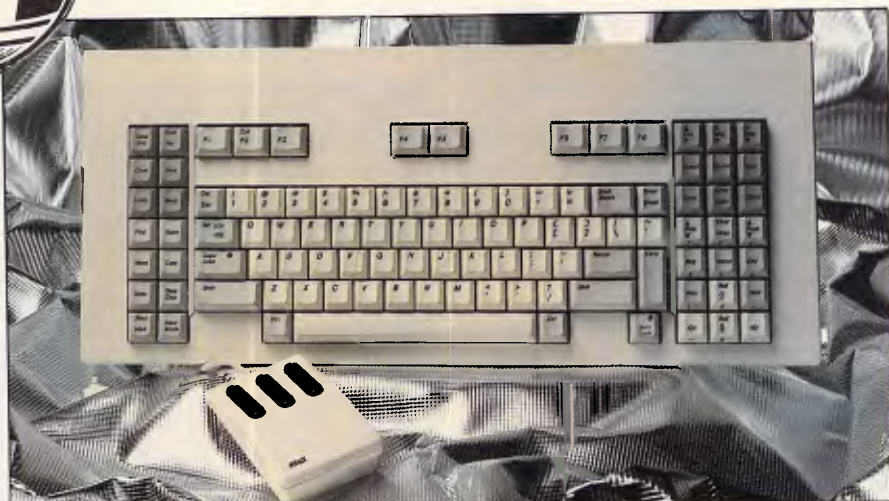
The 103-key keyboard features hard and soft defined function keys
