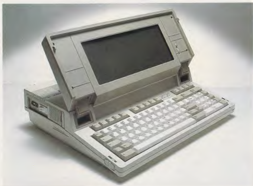
The bulge on the side of the Chendai houses the system's fan
