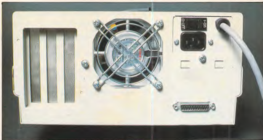
Three expansion slots and a fan dominate Sidecar's rear
