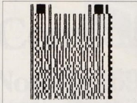
A low-density Softstrip data strip blown up to twice its normal size
